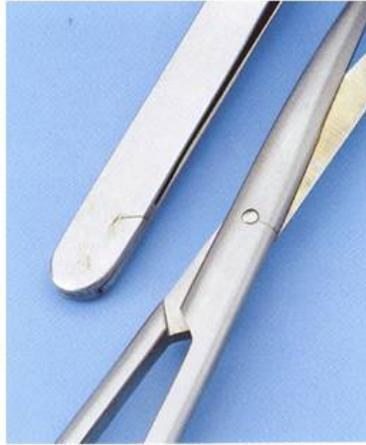
**Stress Corrosion Cracking**
